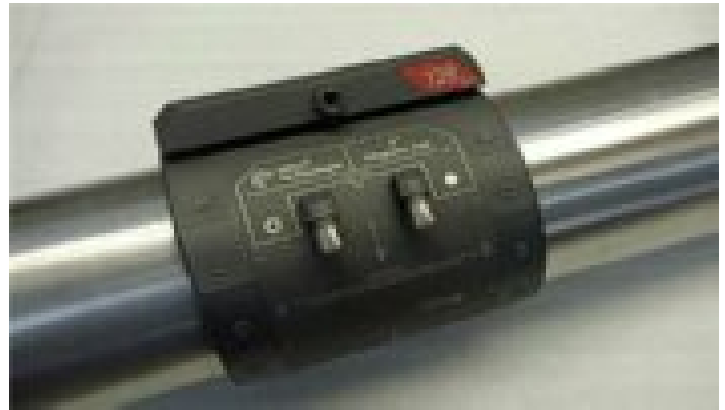
Figure 4: Sonyks Magneto-tool for 100mm/4in diameter pipe and 128kHz test frequency. The tool is lightweight, low profile and can be quickly installed.
